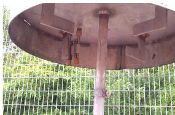
Photograph of a perimeter station and close-up of diffusive monitoring tubes positioned under the steel cap.
