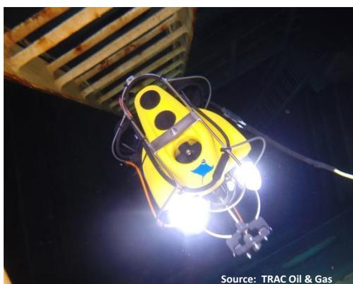
now possible, and remote imaging could be used to undertake these parts of the examination process. The use of remote visual inspection is of particular interest in the high hazard industries, where intrusive human intervention, for example vessel entry, could be reduced.
