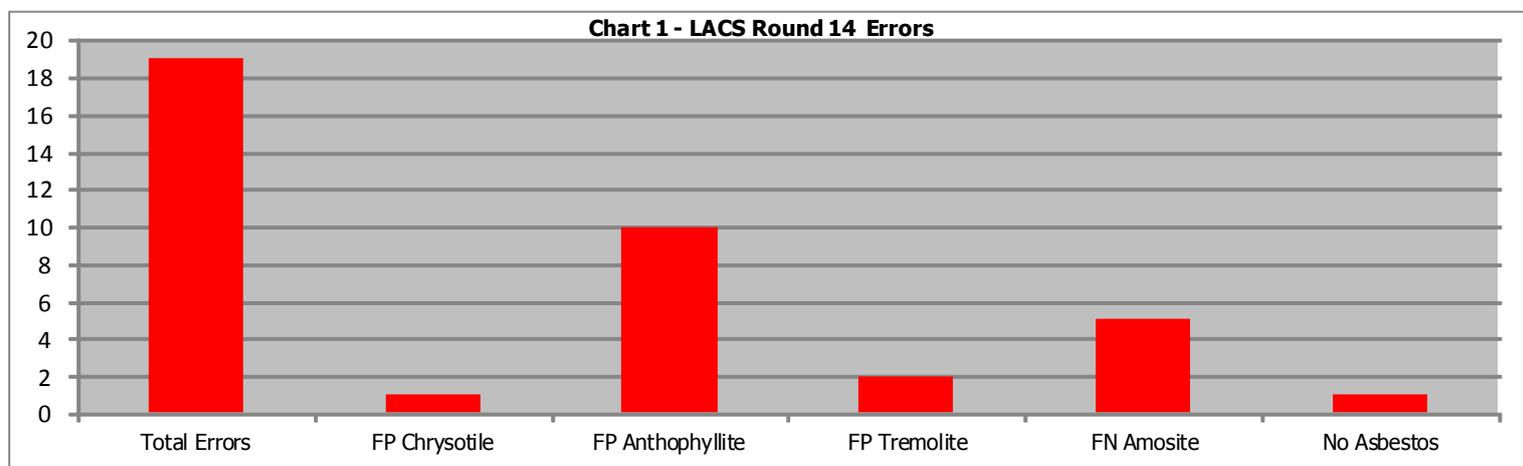
False Negative = Component has been missed. False Positive = Component has been incorrectly identified as present.
