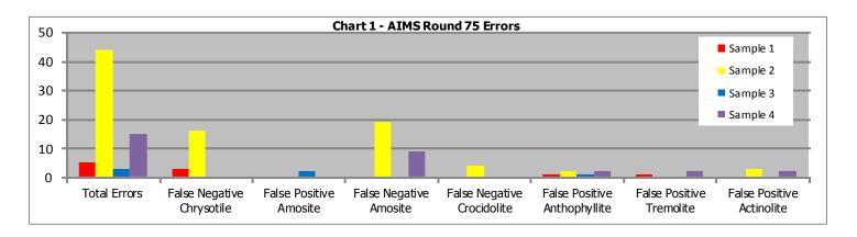
False Negative = Component has been missed. False Positive = Component has been incorrectly identified as present.
