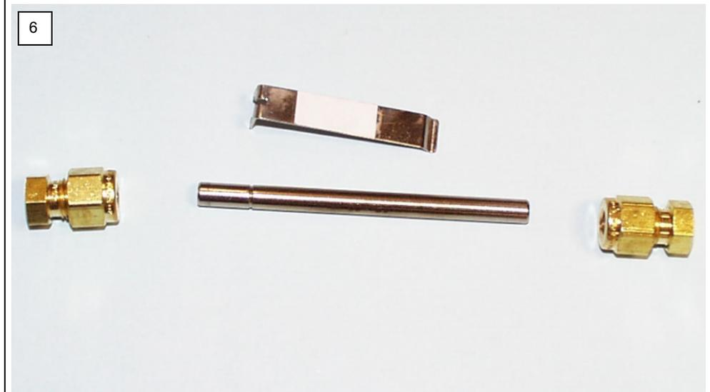
Remove the nuts from the ends of the tube.
