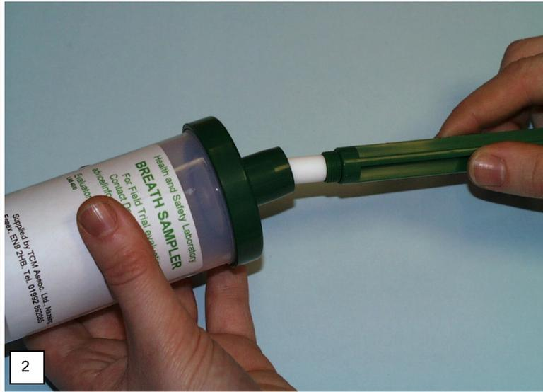
Place the cardboard mouthpiece over the end cap nozzle, and give the sampler to the worker.
