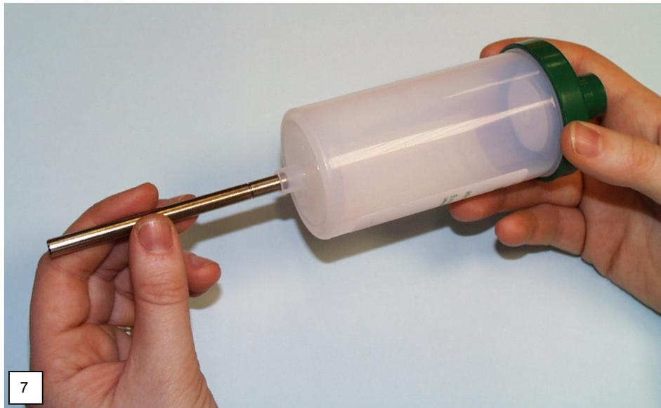
Screw the push rod into place in the end cap.
