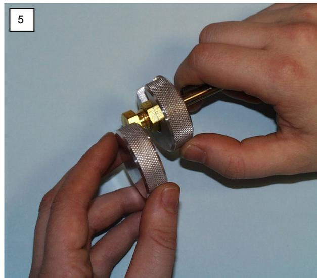
While the worker is giving a sample the stainless steel tube needs to be uncapped. Remove the label clip, if attached. Loosen the gold coloured caps using the Cap-Lok as shown above (by twisting the two discs in opposing directions), then pull the nuts from the ends of the tube.
