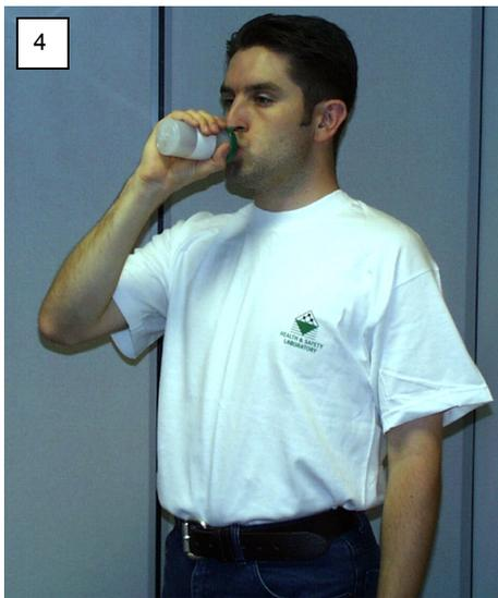
Ask the worker to breathe out through the sampler and encourage the worker to keep exhaling until the lungs are emptied. It is not necessary to breathe in deeply before giving the sample or to breathe in through the sampler.
