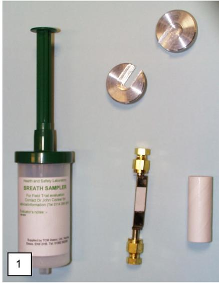
With the pushrod pulled right to the green cap (mouthpiece) end of the sampler unscrew the rod and remove it.
