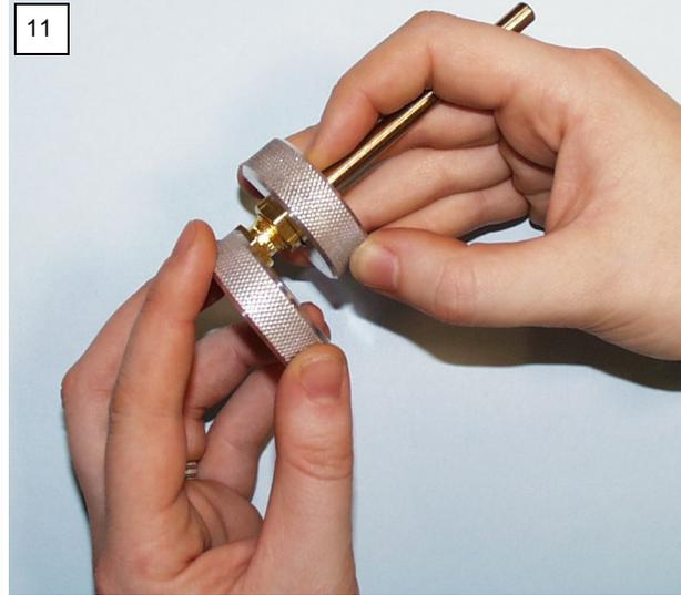
Replace the gold nuts onto the ends of the tube and tighten until finger tight. Use the Cap-Lok to tighten the nut a further quarter turn. Gently pull the caps at each end to ensure they are secure. Attach the label clip and label the tube appropriately.
