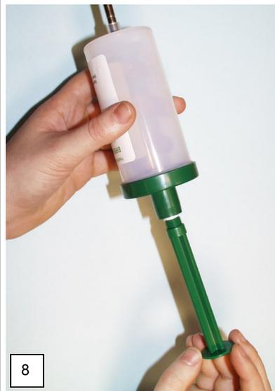
Transfer the trapped breath sample onto the tube by using the push rod to push the piston through the whole length of the sampler over about 10 seconds.
