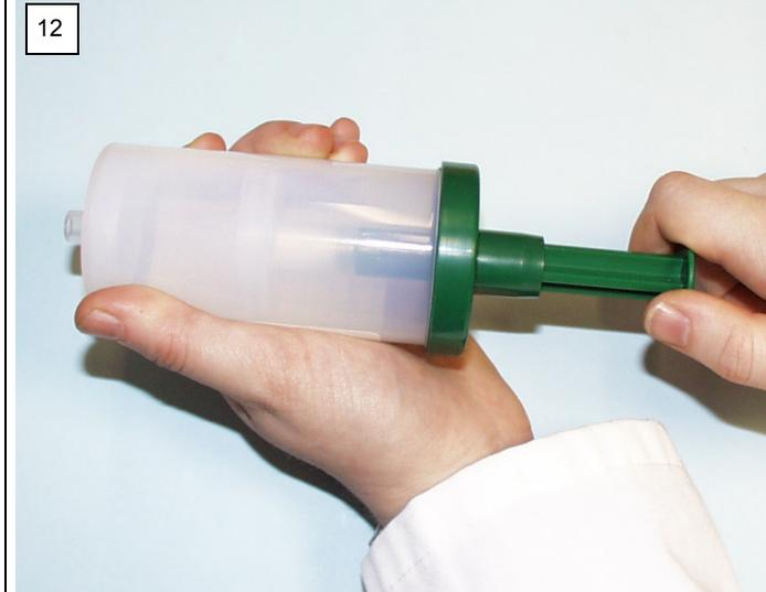
Flush the sampler by pulling and pushing the rod in and out three times. Return the piston to the end cap (mouthpiece) end and detach the rod. The sampler is now ready to be re-used. Repeat the entire process to provide a second, duplicate, sample for the worker.
