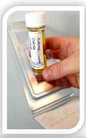
Firmly screw on the cap and place the sample bottle into the protective transporter casing. Ensure that the label details are visible from the outside.
