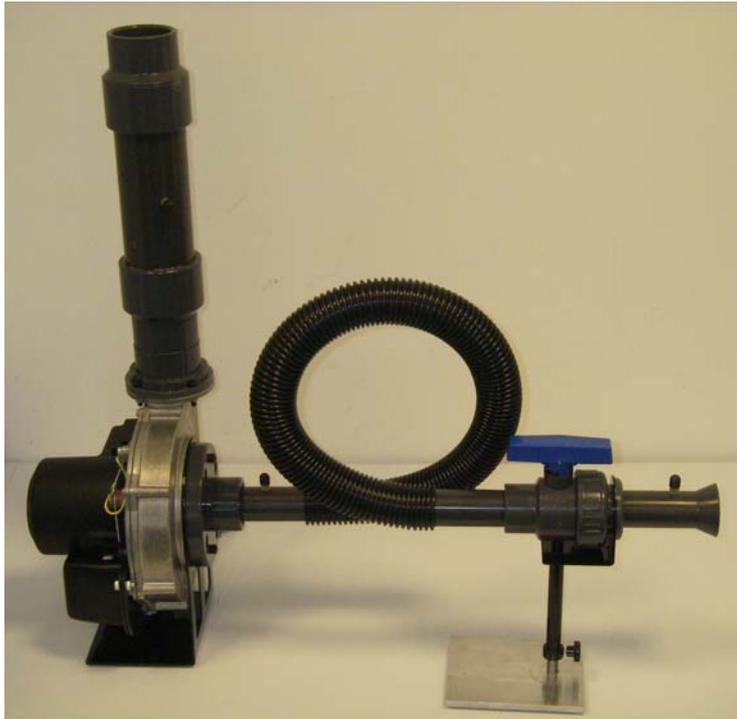
**Figure 4 Possible model set-up for demonstrating how different hoods work**
