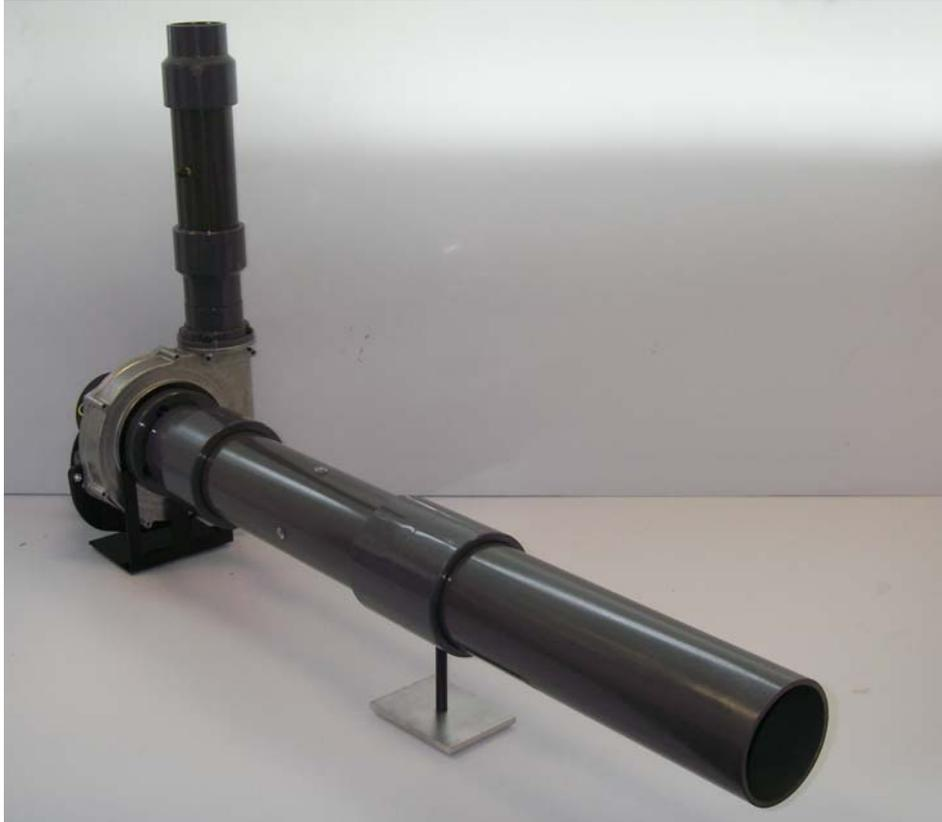
**Figure 5 Arrangement for making duct velocity traverses**
