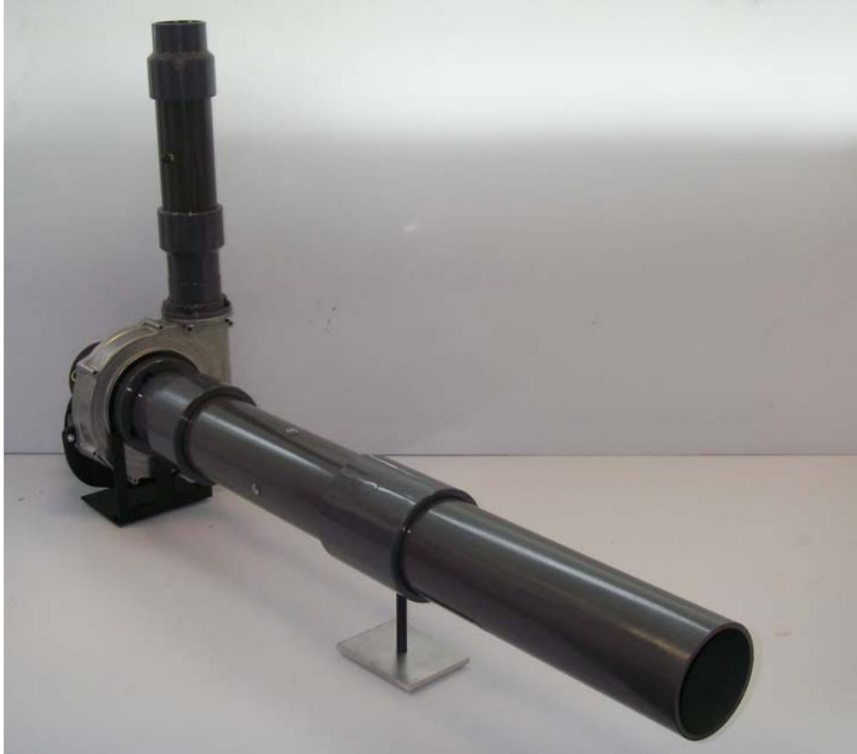
Figure 5 Arrangement for making duct velocity traverses
